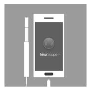
2. Orientate your hearScope™ right side up by pointing it at an object and rotating the hearScope until the image on the hearScope™ application is the right way up.
